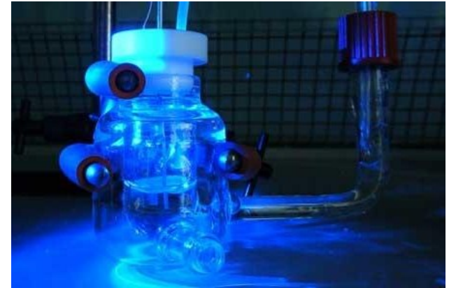
Electrodes in a test cell to produce hydrogen with light. Credit: Dr Erwin Reisner
