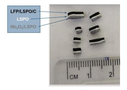
SPS-prepared solid-state batteries with LSPO electrolytes
